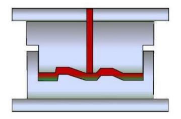
Impregnation of preforms in x-, y- and z- direction
