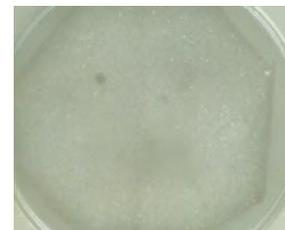
Soiling Test (ISO 846, Method B)
