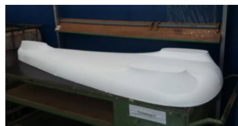
Fig. 3. Plug in polyurethane after machining.
