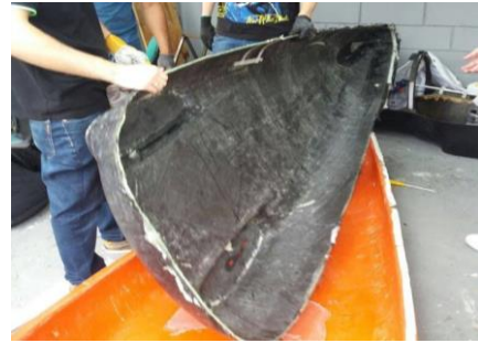
Fig. 5. Composite unibody demolded.
