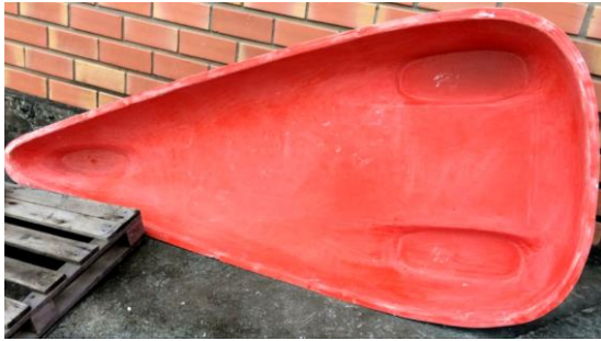
Fig. 4. Mold after spray up process, bottom view
