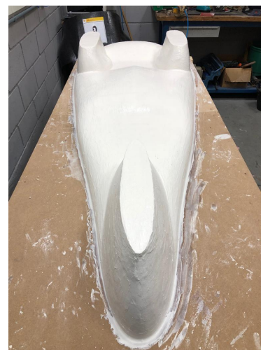
Image 14: New manufacturing method using EPS
