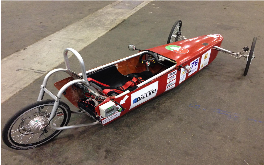
Image 1: Old prototype made of Alluminium and glass fiber
