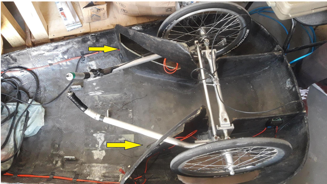
Image 4: The yellow arrows indicate the wheel protection, made from the rear of the old car in image 3.
