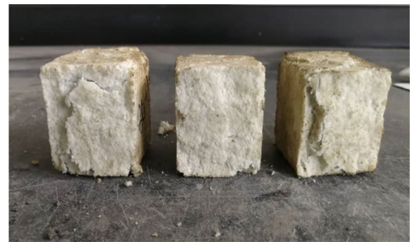
Fig. 4 Compressive strength samples after testing
